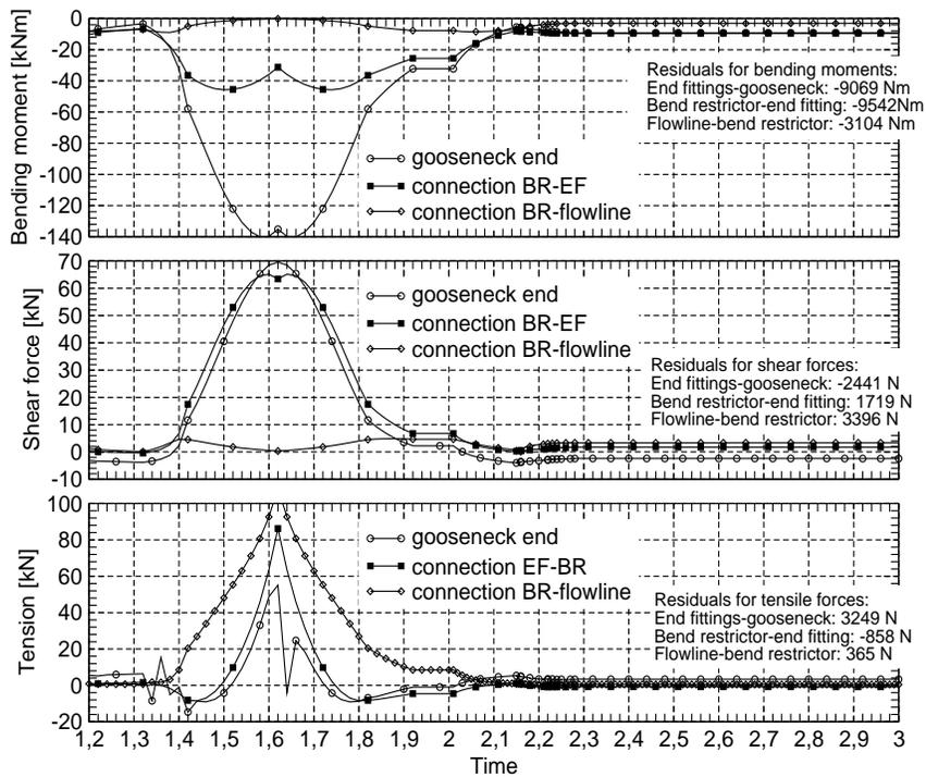
Figure 11: Forces and bending moments at relevant points in the VCM and flowline system (base case).
