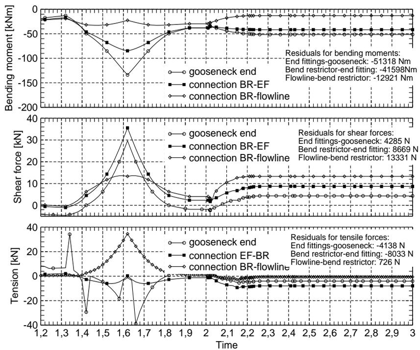
Figure 13: Forces and bending moments at relevant points in the VCM and flowline system (stiffer flowline).
