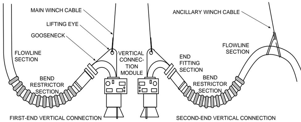
Figure 1: Vertical connection module and flowline termination assembly.
